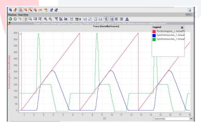
From the scope trace above (zoomed in below), it can be seen that the Knife axis needed to accelerate aggressively to catch up to the sync position yet was sitting stationary for part of the cycle. To reduce wear and tear on the mechanics, it would be beneficial to adjust the sync distance relative to the Master Axis speed to reduce the required acceleration and peak velocity needed for the specific settings.
