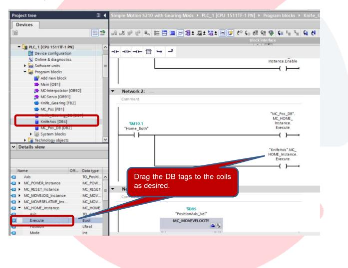
Additionally, an MC\_MoveVelocity block was added to start motion on the Conveyor axis. A Normally Open contact was placed on the Execute and named "Conveyor\_Run". The tag "Conveyor\_Velocity" was added for the commanded velocity and defined as a Global variable. With values "-1" at the Acceleration and Deceleration inputs, the values set up as the default values back at the TO configuration and under Extended Parameters, "Dynamic default values" will be used.
