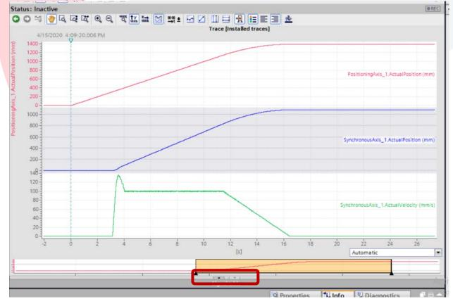
To be critical, and zoomed in, it is shown when the Conveyor (red) is at 400mm the Knife has ramped up, and decelerated back to be at 1:1 Velocity when the Knife (blue) reached 100mm. Also to be confirmed, Knife motion started 100mm before the synchronization location of the Conveyor sync target location of 400mm.
