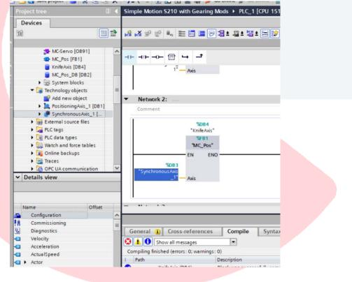
The next step will compile all the existing code and download to the PLC and allow test operation of the second servo axis.
