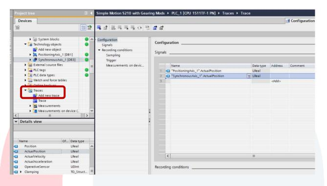
At "Recording Conditions" select "Use max recording duration" and set Trigger Mode to "Trigger on Tag" and select the "Conveyor\_Run" tag used to start the conveyor motion. Set a pretrigger capture to 20 samples, based on OB1 cycle duration.
