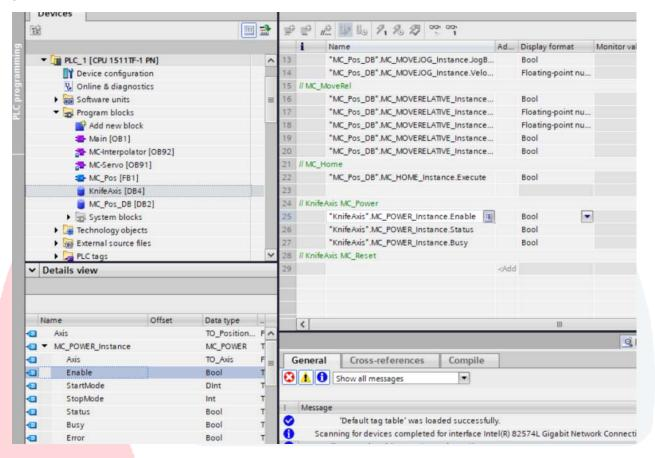
To perform a test jog, click on the "Monitor All" icon. Place a "1" (True) at MC\_Power Enable. Send that to the PLC using the "Modify All" icon. MC\_Power Enable is necessary first since many motion operations, like Jog, trigger on the rising edge of an Execute input. Check mark next to Modify Value column is important. Only items with the check mark will be modified by the next Modify All. The "exclamation point warning" indicates the value is only sent with the next Modify All trigger.
