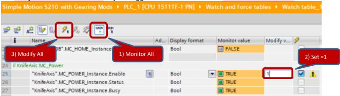
Next put a "1" at "MC\_MoveJog...Forward" and put 50 (mm/sec) as a "KnifeAxis MC\_MoveJog ...Velocity". Follow with clicking on "Modify All" icon. The KnifeAxis should be rotating. To stop the Jog, put a "0" (False) in for MC\_MoveJog...Forward" and trigger "Modify All". Next set MC\_Power to "0" and "Modify All" again to disable the axis.
