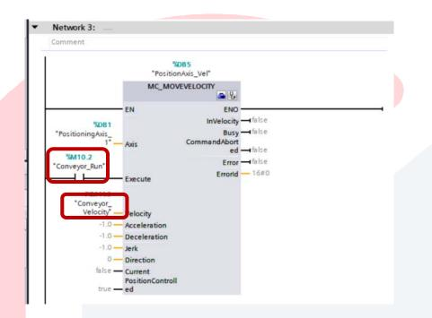
Unique to a PLC Open type Velocity moves, the motion will begin on the rising edge of the Execute input, but the axis will not stop the velocity move when the input goes away. Instead, an MC\_Halt can be used to define a deceleration and stop motion. Shown below a normally closed contact of the same input used to start the velocity move is used to trigger the stop using the MC\_Halt brought over from axis DB tags.
