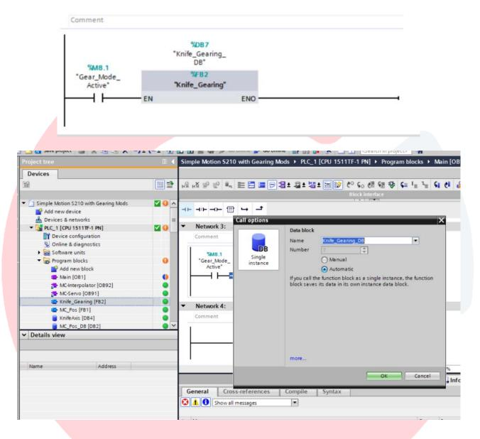
Download all changes to the PLC. With major changes a PLC Stop will be required. Confirm the PLC is started following the Load.
