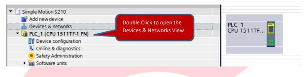
In the Devices and Networks Window, Drag and Drop in your S210 Drive model from the hardware catalog.
