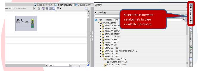
This will be the second S210 drive in the hardware configuration so name that drive "Drive2" by clicking on the default drive name given in the Network View where the drive is dropped into the project.
