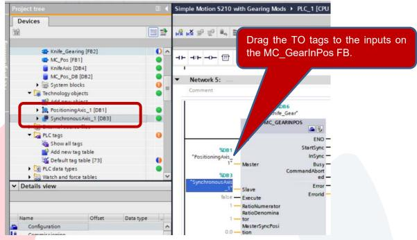
Position synchronized operations will require both axes to be "Homed" initially. To simplify operation, add a network to "Enable" both axes and a network to "Home" both axes in this function block as shown below.
