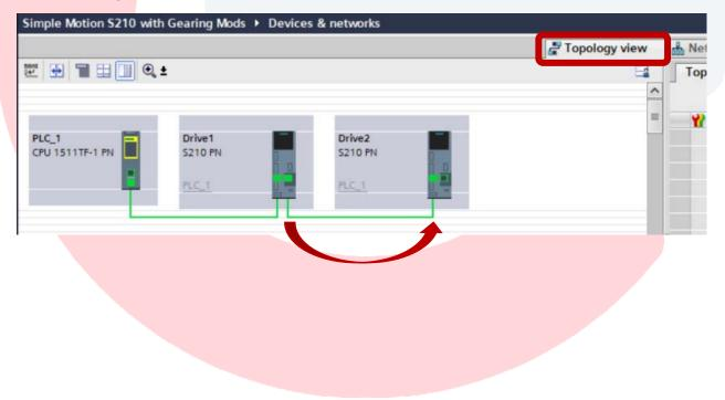
The next steps establish the IRT relationship and timing. This was covered in detail in the "S210 Simple Motion" app note, so will only be covered in bullet points here.
