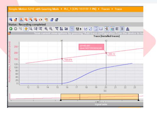
To illustrate a Conveyor velocity 10x faster and the relationship of SyncProfileReference=1 versus 0, it would be expected to allow the Knife axis more "distance" to come up to speed and catch the Conveyor, since it was already at about twice the 1:1 speed to catch the Conveyor at the slow conveyor speed. With SyncProfileReference=1, this synchronization is based on the user defined distance. If
