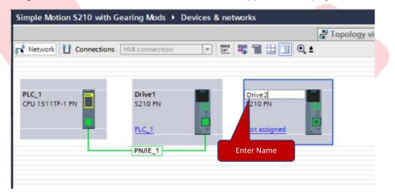
This drive should have an X150 address 192.168.0.3 so click on the icon to display the IP addresses and then by clicking directly on the displayed address, change the address as desired. Do not modify the 169.254.11.22 address; this is the Siemens service port default address for Port X127 on Sinamics drives.
