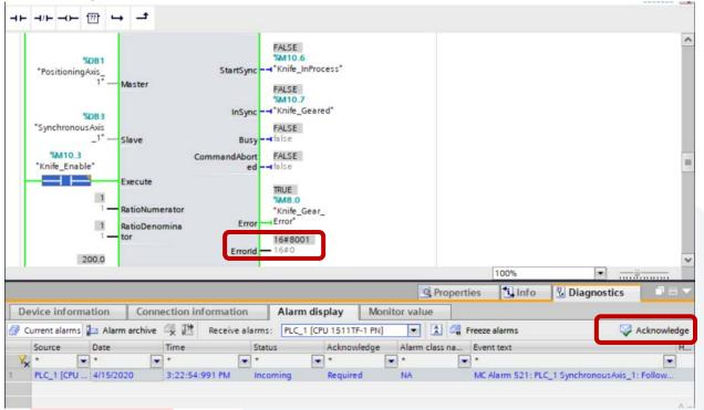
In order to track down a Technology Block error (which is not reported as a Hardware fault) one needs to observe the Error ID reported from the effected Technology Block, select F1 Help while having Focus on that Technology Block and reference the information in the related Help description or additionally, follow the link to the decoded error codes as shown below with Error ID of (Hex)8026 displayed:
