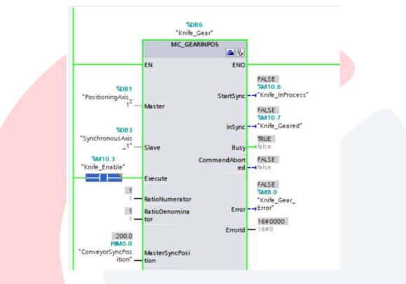
Next, set a relatively low velocity for the "Conveyor" and trigger the "Conveyor\_Run" input knowing this will also trigger the Trace to begin recording the two servo axes Actual Positions.
