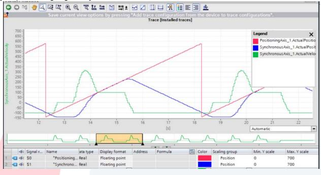
One more useful tool is the use of the measurement cursors in the menu bar, which can either be positioned by dragging the lines to desired locations, or if there is a known specific location they should be at, at the right, the desired locations can be manually typed in and the cursors will move to that location. Below, "Horizontal Measurement Cursor" positions are placed at 200mm and 300mm to confirm the 1 to 1 synchronous segment.
