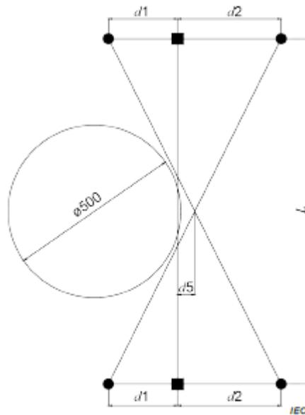
**Figure D.19 – Positioning of the muting sensors**
