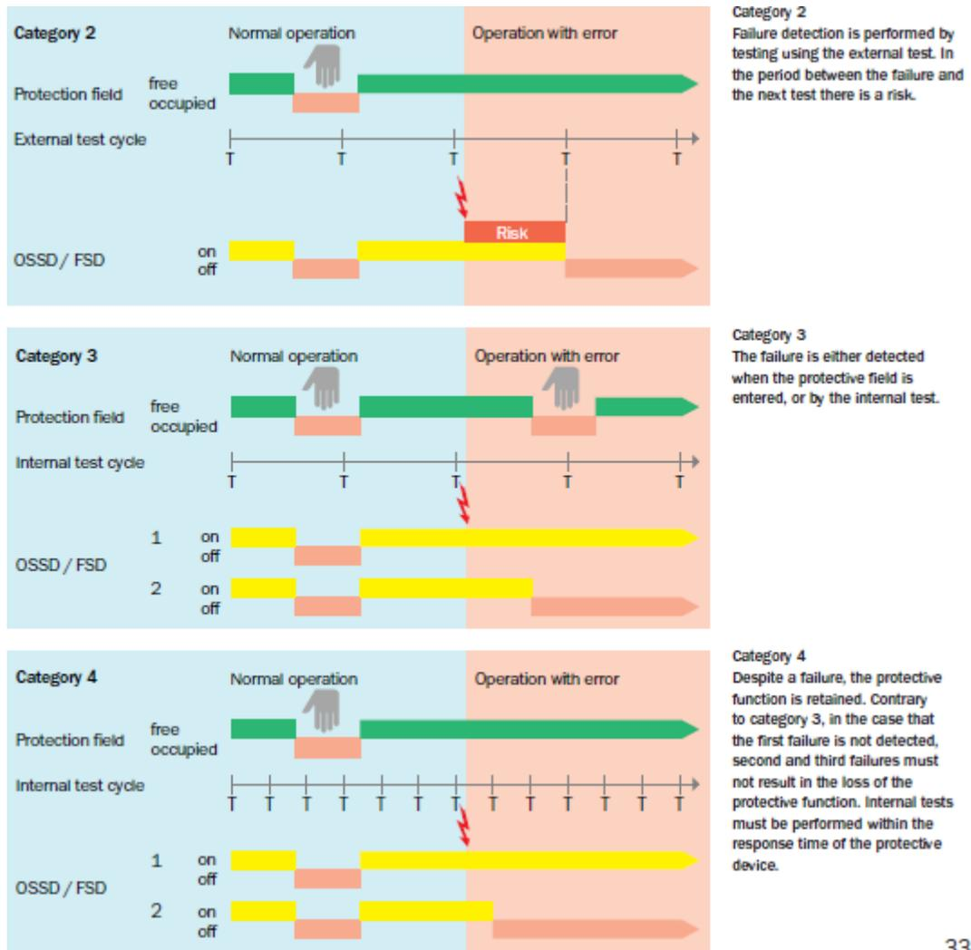
Figure 1 - ESPE Types (courtesy of SICK AG)
