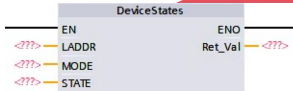
The DeviceStates instruction can be found in the Instructions task card in the Extended Instructions section, and under the Diagnostics folder. You can view the help at any time by single clicking on DeviceStates, wait a few moments for a tool tip to appear, and then click in the link to display the online help. Once you have added the DeviceStates instruction to a network, it can be found in Program Blocks\System Blocks\Program Resources folder for future use.
