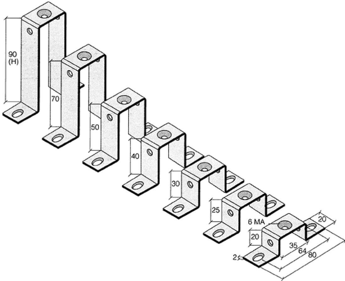
Top hole tapped (M6), side holes unthreaded, bottom mounting holes oblong.
