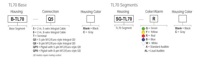
Select the 5-pin base for tower light configurations of up to 4 modules. Select the 8-pin base for tower light configurations of up to 6 modules.
