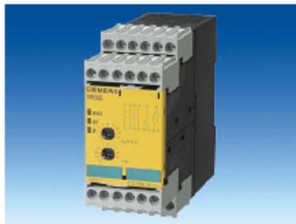
SIRIUS SAFETY RELAY FOR SAFETY-ORIENTED STANDSTILL MONITORING, 24V DC, 45.0MM, SCREW TERMINAL, FK INSTANT: 3NO 1NC, FK DELAYED: 0, MK: 3, AUTO START, BASIC UNIT, MAX. ACHIEV. CAT. EN954-1: 4, MAX. ACHIEV. SIL TO IEC61508:3.
