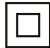
“Double insulation” symbol (protection class 2)
